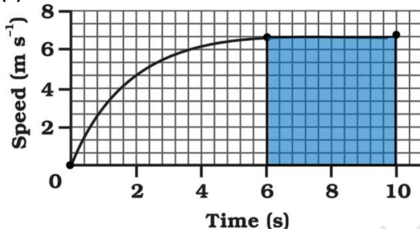
The part of the graph in red colour between times 6 s to 10 s represents the uniform motion of the car.
