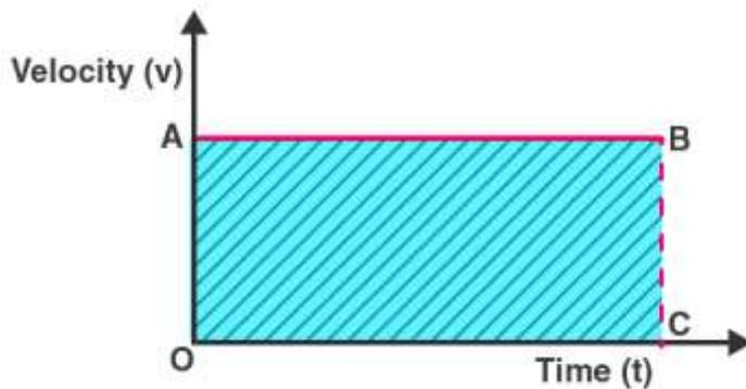
**Ans:** The area beneath the velocity-time graph corresponds to the area of the rectangle OABC, calculated as OA multiplied by OC. Here, OA represents the object's velocity, and OC indicates time. Thus, the shaded area can be expressed as:
