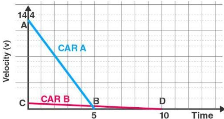
The total displacement of each car can be determined by calculating the area under the speed-time graph.
